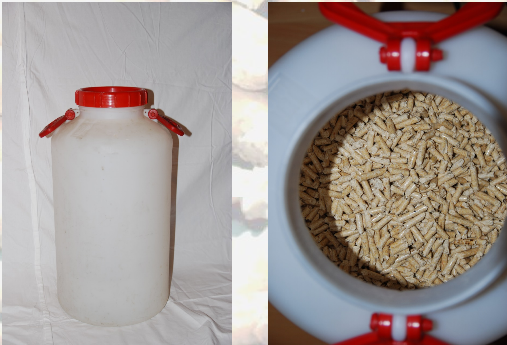
Fig. 1: 25 Liter polypropylene drums filled with common-use wood pellets used for series 1. Source: Pyrek, 2014
