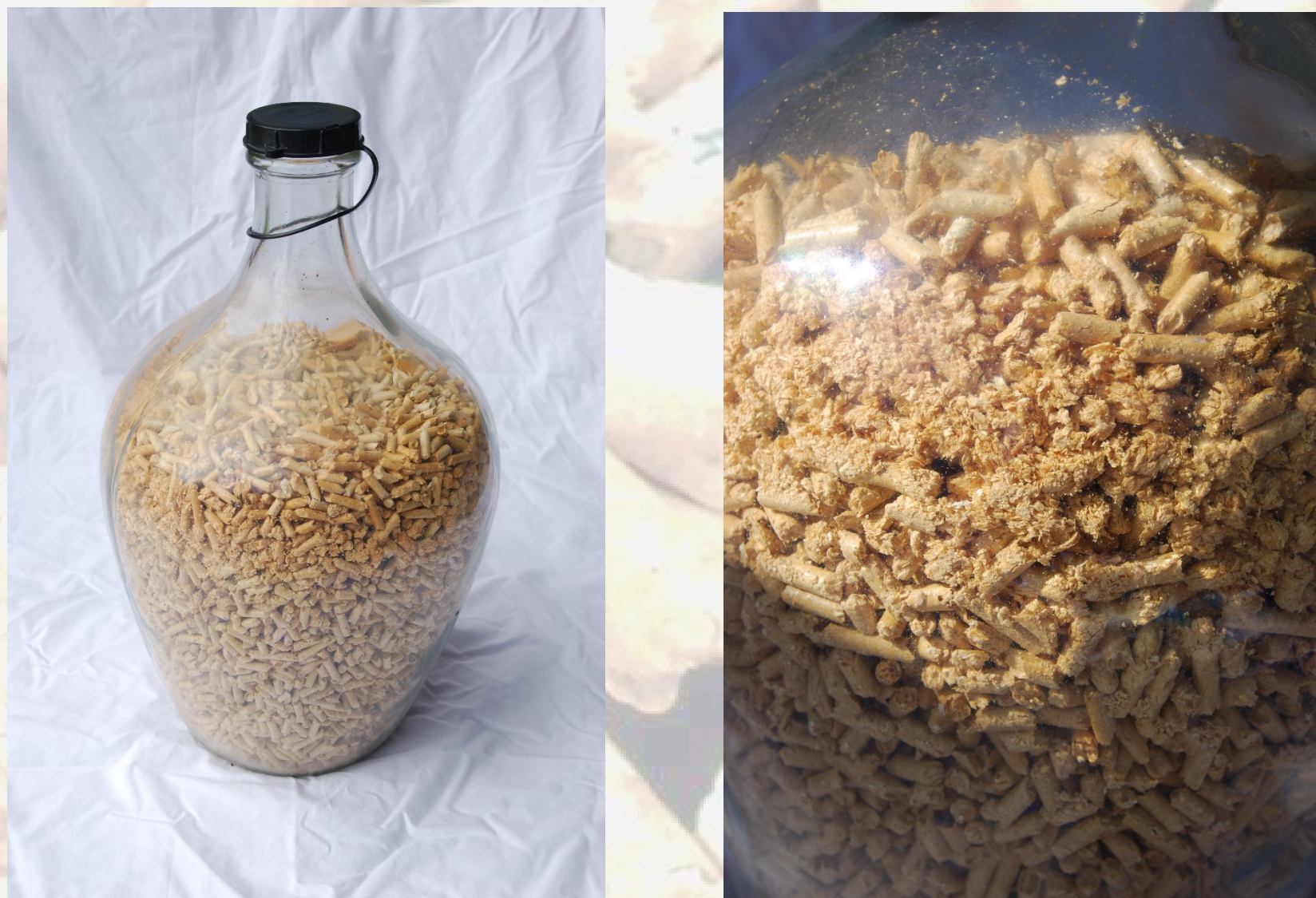
Fig. 2: 15 Liter glass container filled with same common-use wood pellets as used for series 1. The right picture shows a remarkable degradation of the material Source: Pyrek, 2014
